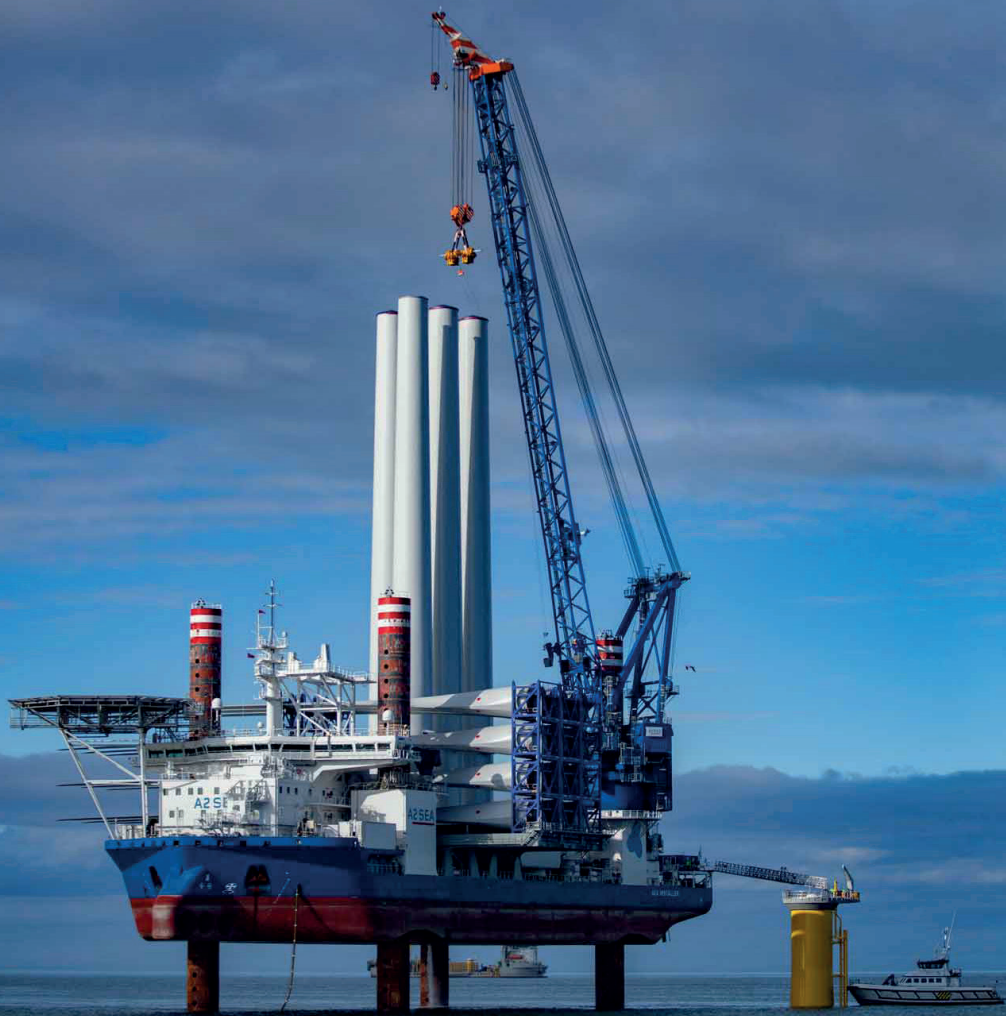
An installation ship holds blades and towers ready to be built. Photo: Ørsted.
